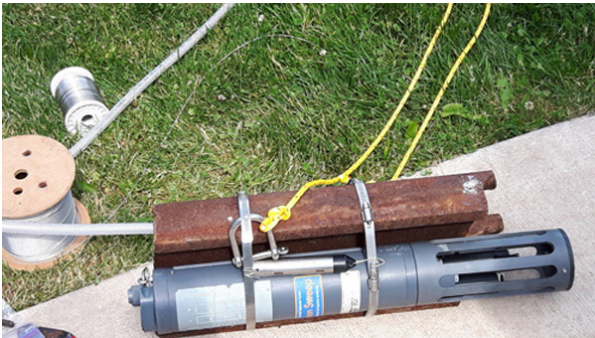
This monitoring unit measures multiple water quality indicators.
